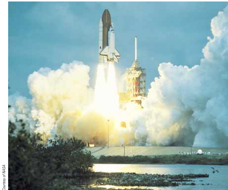
Figure 9.27 At liftoff, enormous thrust is generated by the space shuttle's liquid-fuel engines, aided by the two solid-fuel boosters. This photograph shows the liftoff of the space shuttle Columbia , which was lost in a tragic accident during its landing attempt on February 1, 2003 (shortly before this volume went to press).
